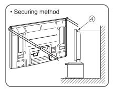
Use strong wire or chain which is commercially available to secure the plasma television to a solid area of the wall or a pillar.
