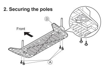
Use the assembly screws  $\widehat{\mathbb{A}}$  to secure the poles firmly to the bottom of the base.
