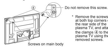
Remove the screws at both top corners on the rear side of the plasma TV, and attach the clamps 4 to the plasma TV using the removed screws.
