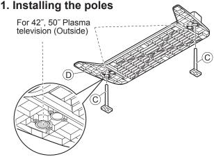
Insert the poles  $\bigcirc$  into the left and right holes in the underside of the base  $\bigcirc$  so that they fit securely as shown in the illustration above.
